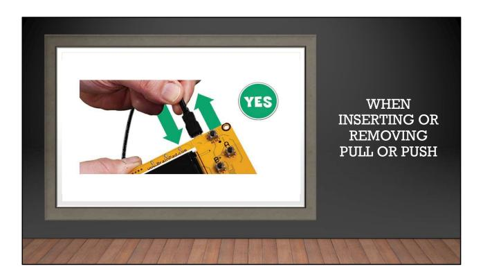
When connecting the BrainPad to a compute we use a microUSB cable. The USB cable should always be pushed or pulled straight in or out.
