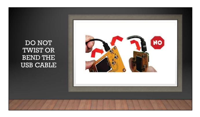
Never twist or bend the cable sideways when removing. This could break off the connector, breaking your BrainPad.
