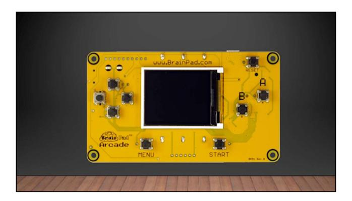
Let's add our first game to the BrainPad. First, we need to tell the BrainPad it's time to LOAD a program. The first time you plug in a USB cable you may see the bootloader screen already. If you don't then you can put the BrainPad into loader mode by pressing the RESET button for a moment until you see the LOADER SCREEN and the LED turns RED. Your BrainPad is now ready for a new game.
