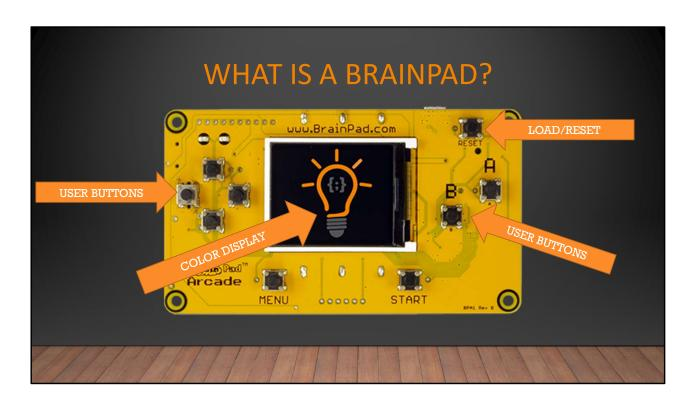
A BrainPad is a circuit board designed to spark a person's knowledge to learn coding and electronics. 1 & 2. On the front we have USER BUTTONS. These are used to run the programs we create and load. 3. The BrainPad is equipped with a color display. The games you make will appear here on the color screen. 4. Load and Reset button. This button is used to restart the BrainPad and to put into a mode that we can add our programs, more on that later.
