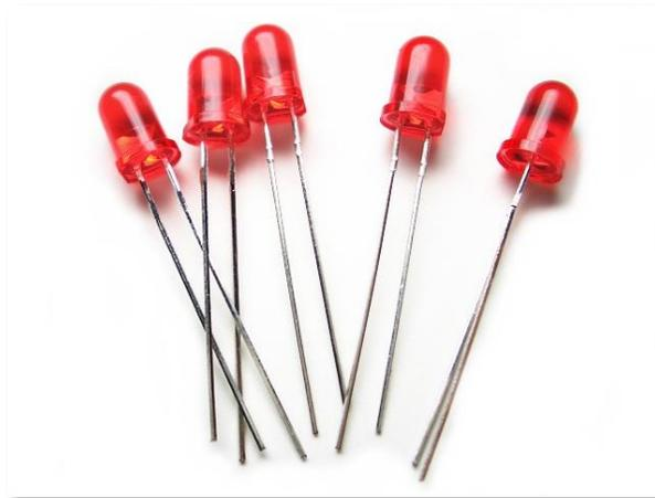
LEDs are very inexpensive and come in different colors. They have two leads where one should be longer than the other. Some LEDs have more than one color (like the BrainPad's Light Bulb.) We are not covering those LEDs. To control an LED a current-limiting resistor is needed. Some common values are 220, 330, or 470 ohms. You will also need some wires and a breadboard.
