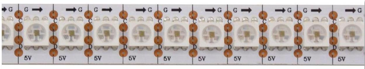
The strip can be cut to any needed size. To keep my setup from drawing too much power, I will cut it down to 25 LEDs. Now to soldering some wires. The arrow on the strip needs to point away from the side you solder the wires to. The 4 wires are G-Ground, C-Clock, D-Data and 5V.
