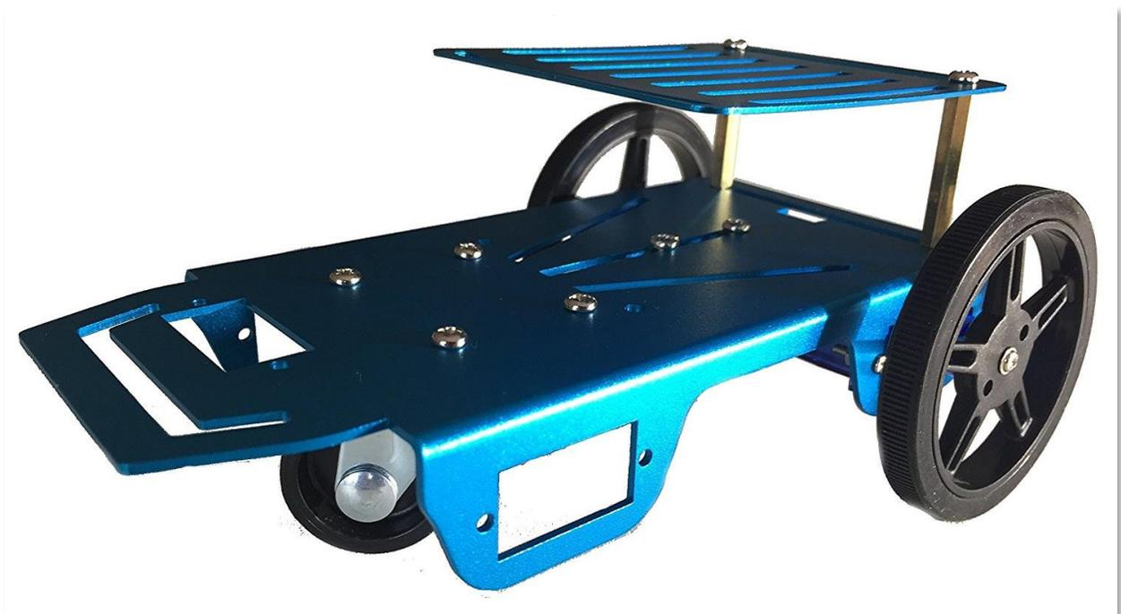
Here is where things got a bit tricky! The robot comes with wheels and motors. The motors look like servo motors, but they turned out to be not servos, just regular motors. I could tell because they only had two wires instead of
