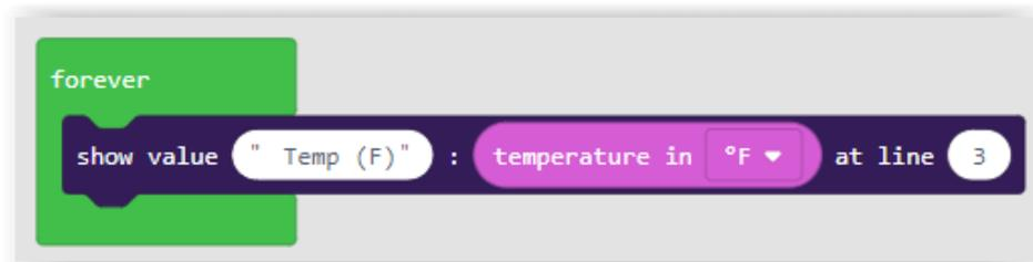
So far, we have made a thermometer that will display the temperature on the BrainPad's display. Now we must convert the temperature into an angle and send it to a servo motor to move the dial on our thermometer. Let's make our thermometer work over a range of -20° Fahrenheit to 120° Fahrenheit.
