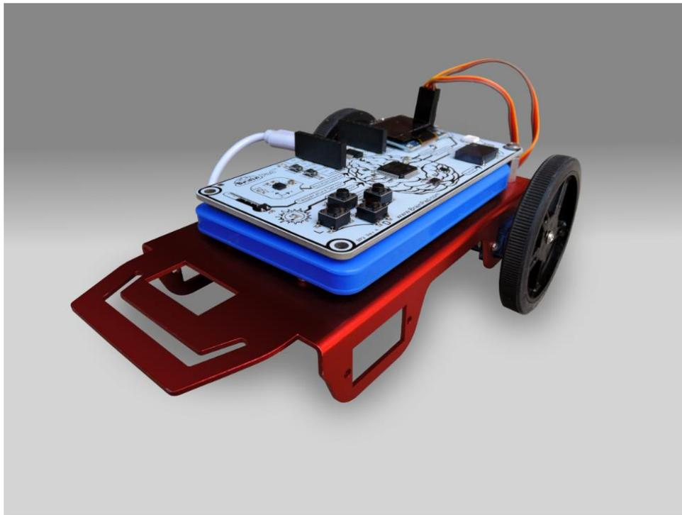
This robot is finally ready to dance! To go forward, both motors need to turn forward. However, as one of the motors is facing right and the other is facing left, one will have to turn opposite from the other for the wheels to
