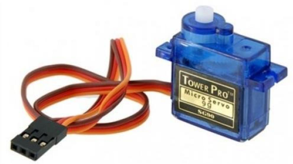
Servo motors (or servos) are often used in radio-controlled models and can be found online and at local hobby stores. These servos draw power from the BrainPad, which in turn draws power from your PC or a battery. Therefore, we recommend using the smaller servos, called micro servos. Some of the larger servo motors draw too much power to work properly without adding an additional power supply.
