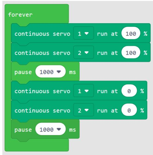
If the motors continue to turn when the speed is set to zero they need calibration. Most servo motors will have a tiny adjustment inside. You will need a tiny screwdriver for this task.
