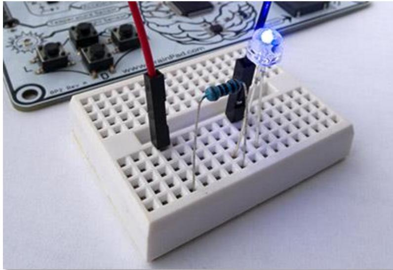
If you have a circuit that you would like to make more permanent, there are several options from easy to use pre-made prototyping boards to designing your own circuit boards. Circuit board designs can be drawn by hand or drawn using free computer-based design tools. This is what makes the BrainPad so special – it is simple to get started, but you can advance as far as you like while learning at your own pace.
