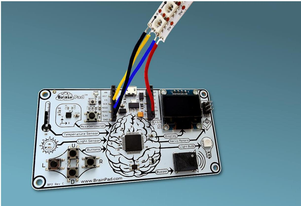
Each LED has three internal LEDs. They are red, blue and green. By controlling the levels of these base colors, you can create any color you wish. There are several online tools to help with color picking. A good example can be found at <http://www.rgbtool.com>. What you care about are the R, G, and B values.
