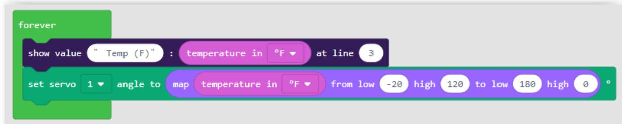
You will notice that the angle goes from a low of 180 to a high of 0 in our map block. Isn't this backwards? The reason is that when the servo motor is set to 0 degrees the motor is turned to the right, and when the servo is set to 180 degrees it is turned to the left. Mapping the temperature of -20° Fahrenheit to 0 degrees on our servo would make the thermometer read backwards.
