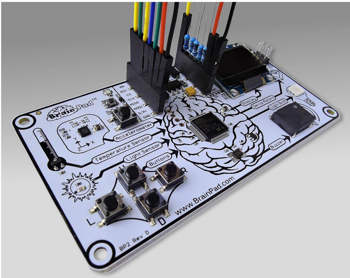
As mentioned in the first chapter of this book, there are multiple ways to expand the BrainPad, thanks to the female headers located near the USB connector.
