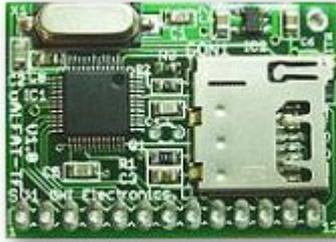
μALFAT-TF is an OEM board of μALFAT™ chip with TransFlash (micro SD) card connector. It has very small dimensions which makes it ideal for small data logger. This OEM board is one of the smallest OEMs with high performance file system abilities , about 1" by 1.4"!
